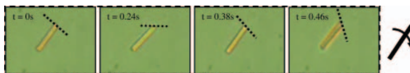
Figure 2. Snapshots of glass cylinder dispersed in calamitic nematic liquid crystal, ZLI 3640, at different time steps with dc field amplitude: E \approx 1.0 \text{ V } \mu\text{m}^{-1} (12 \mu\text{m} cell with 6 \mu\text{m} spacers). Pictures were taken between uncrossed polarizers. The rotation around the long axis of the molecules can be seen by following the rotation of the direction of one of the edge (indicated by dotted line to guide the eye) that is slanted with respect to the long axis.
